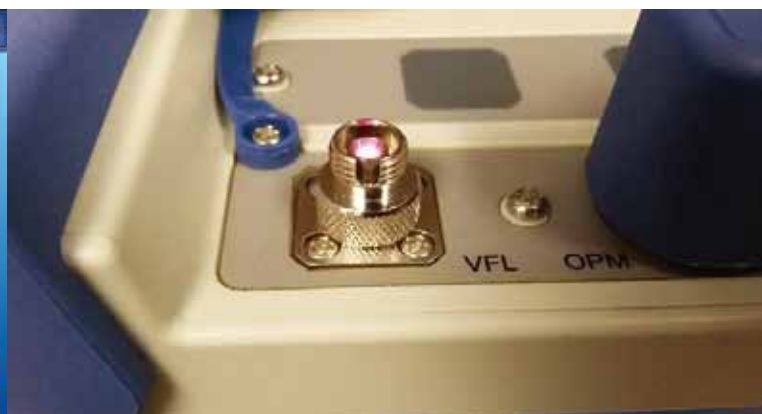
Pictured: Visual Fault Locator (VFL) beam illuminates bends, splices, and faults in optical fibers.
