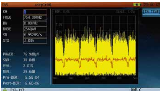
Figure 11: The EVS time-domain function is used to locate signatures of LTE interference signals under a QAM carrier - without interrupting service.
