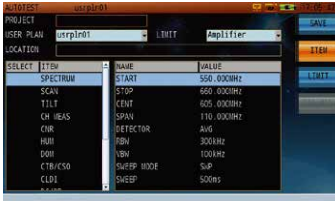
Figure 25: Define limit profiles to perform auto tests. Results will show Pass or Fail according to channel plans & limit profiles, eliminating the need for interpretation.
