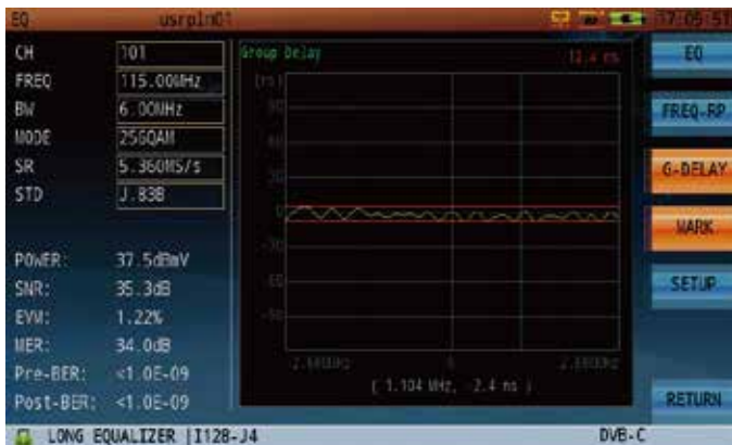
Figure 15: Group Delay is also derived from the adaptive EQ power coefficient. Group delay should not exceed 200 ns/MHz (upstream) or 75 ns/MHz (downstream).
