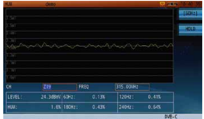
Figure 8: The Digital Hum measurement can detect changes in modulation amplitude - typically due to powerlines.
