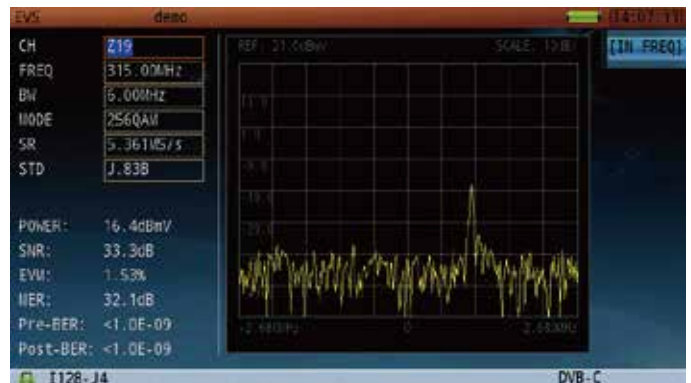
Figure 12: The EVS frequency-domain function measures interference signals under a QAM carrier.
