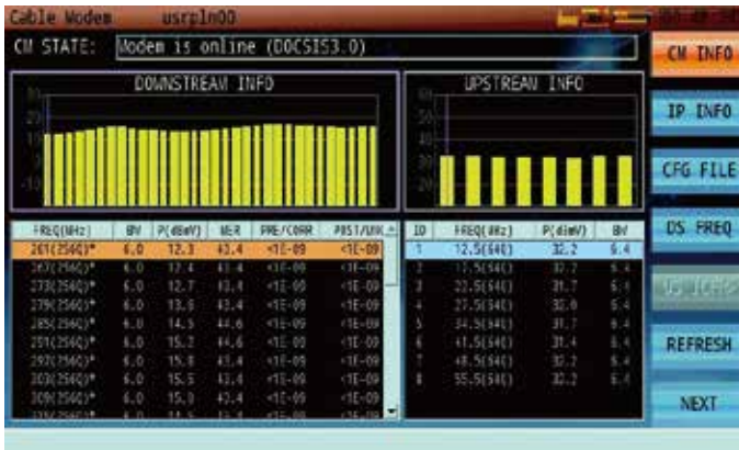
Figure 19: DOCSIS 3.0 32x8 Cable Modem Analysis
