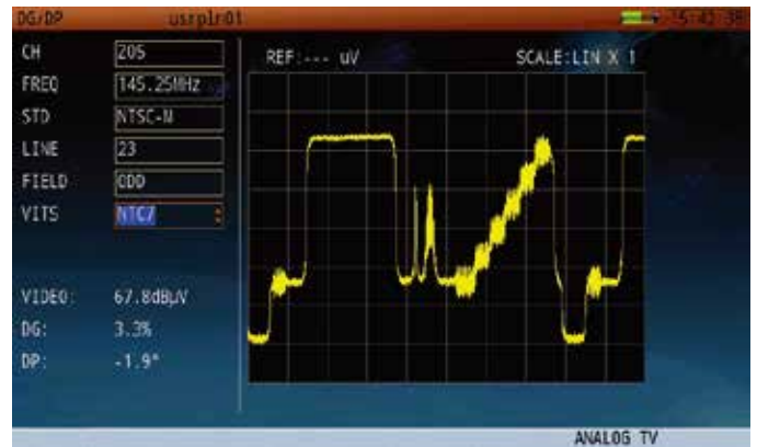
Figure 6: Use VITS and Analog TV Gated Mode to measure analog TV video parameters without interrupting service.
