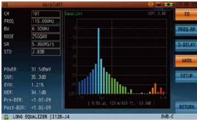
Figure 13: The Adaptive Equalizer uniquely compensates for linear distortions such as phase noise, impedance mismatch & group delay, in the HFC network.
