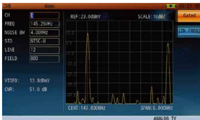
Figure 5: Analog TV Gated Measurement supports in-service CCN, CSO, CTB, CLDI, DG/DP, DOM and ICR measurements.
