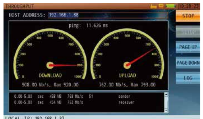
Figure 24: The IP test suite includes tests such as Ping, traceroute, and FTP download/upload.
