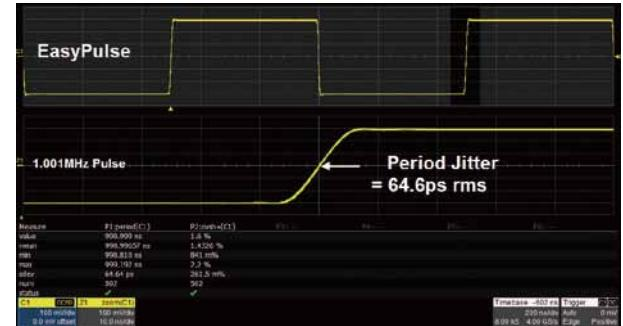
When a Square/Pulse waveform is generated by DDS, there will be a one-clock-jitter if the sampling rate is not an integer-related multiple of the output frequency. SDG2000X EasyPulse technology successfully overcomes this weakness in DDS designs and helps to produce low jitter Square/Pulse waveforms.
