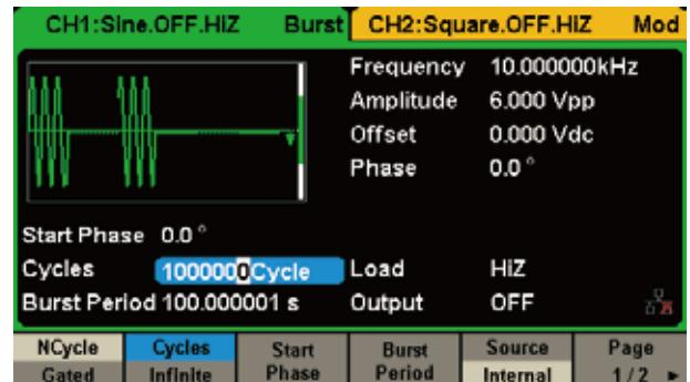
SDG2000X supports two Burst modes, "N cycle" and "Gated". The Burst source can be configured as "Internal", "External" or "Manual".
