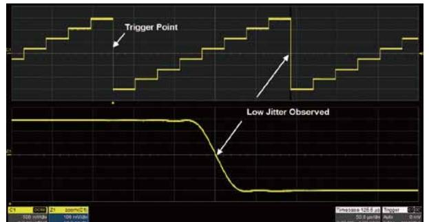
TrueArb generates arbitrary waveforms point by point, never skips any point so that it can reconstruct all the details of the waveform as defined.
