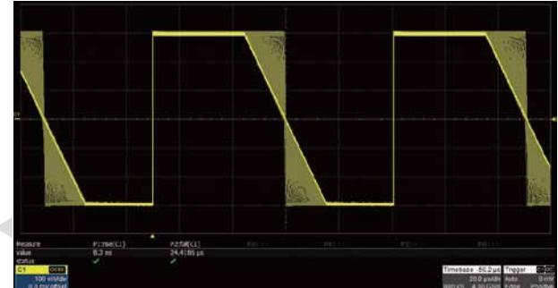
The Pulse width can be fine-tuned to the minimum of 16.3ns with the adjustment step as small as 100ps.
